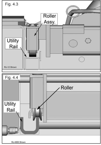
6. Ensure that the Utility Rail Channel is clean of debris, tools etc.
