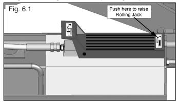
Under certain circumstances it may be necessary to prime the Air Hydraulic Pump Unit. Refer to the manual that came with the pump for these instructions.
