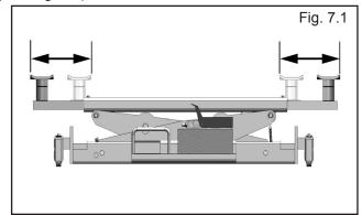
7. Raise the Rolling Bridge Jack by pushing on the Raise end of the pedal of the Air Hydraulic Pump. Keep an eye on the jack as the lift pads make contact with the vehicle to ensure that proper contact is maintained as the weight of the vehicle is supported by the Jack.
