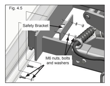
8. Repeat the process for the other Rolling Bridge Jack if installing in pairs.
